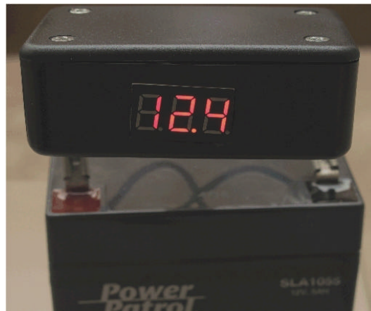
Figure 1: The EZ-Volt Meter Measuring a 12 Volt SLA Battery
