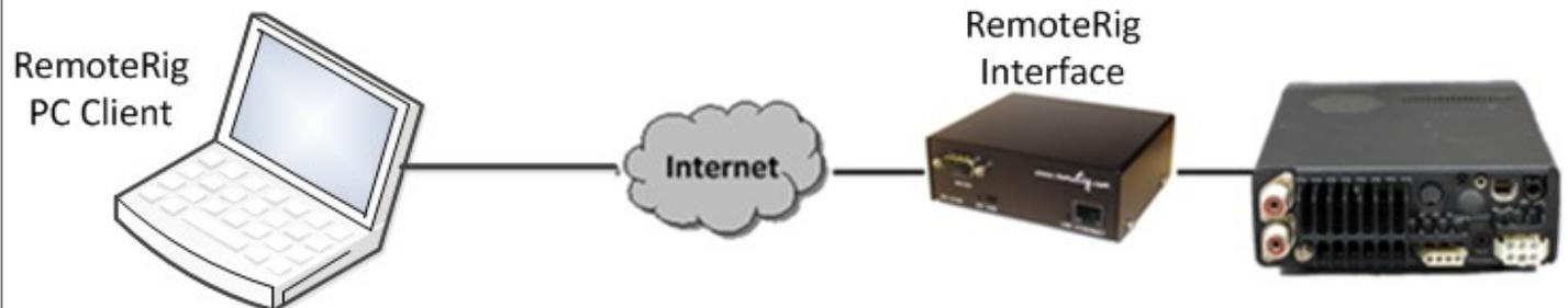
separate audio connections for transmit and receive audio may also be made to the “black boxes” and packetized for transmission over the internet. Because of the wide variety of radios this application is suited for, setup can be a bit more complicated than the Icom RS-BA1 solution. However, once it’s set up, it’s very portable and results in an operation that looks like a ham radio at the remote end.
